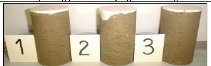
The change of sound degree for specimens in repeating process of drying and wetting.
